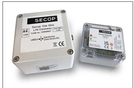
Fig.3 Size comparison of previous (left) and new (right) Secop Gateway
